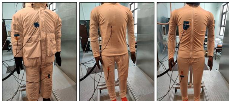
Fig 1 ECWC layers worn on Newton thermal manikin with thermocouples
